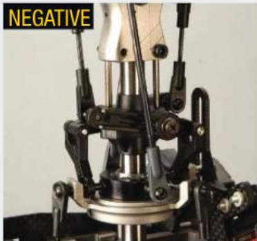
The Thunder Tiger Raptor is a mechanical pitch helicopter that uses separate servos for each function.
