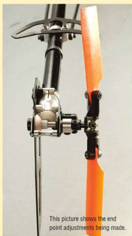
Don't allow the tail blades to over rotate or they can lock up in flight and cause an out of control piro rate.
